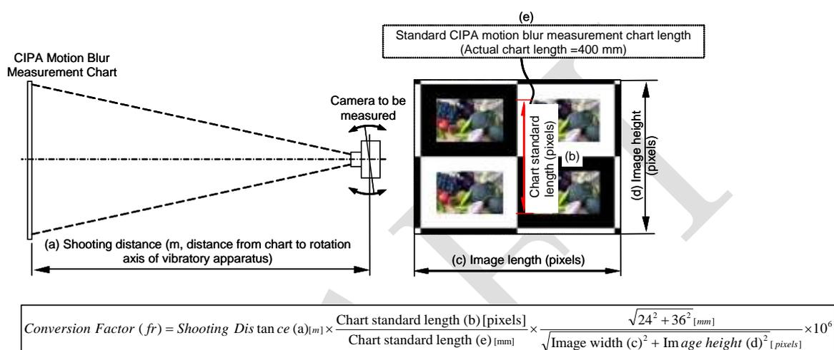
Figure 5-4-1: Method for calculating conversion factor (fr)
