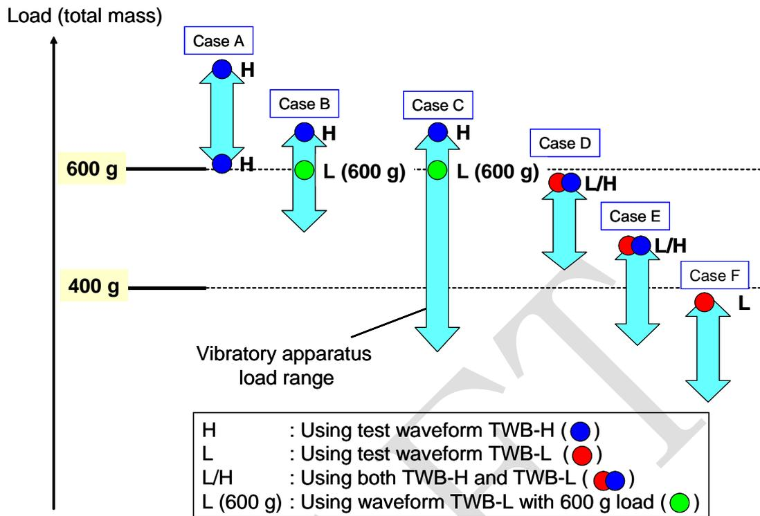
Figure 5-2-3c: Test waveform and load combinations
